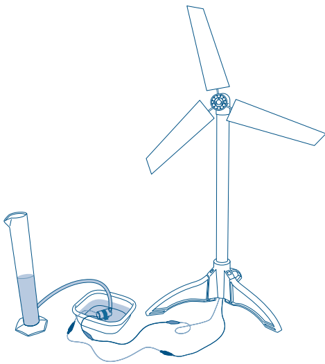
Wind Turbine and water pump
